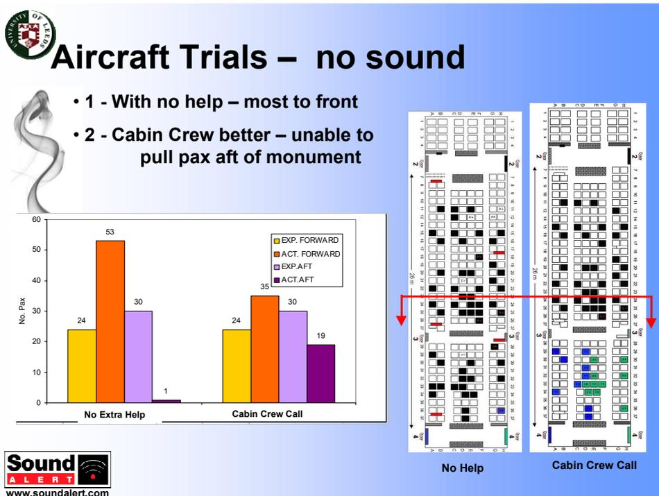
Figure 2. Data from the trials where directional sound was not used. The bar graph on the left shows the expected (exp.) and actual (act.) door usage. The schematic drawings on the right show the actual exits used by each passenger. The exits are colour coded. Black = front right exit; blue = rear left exit and green = rear right exit. Note the only passenger to use a rear exit in trials 1 used the left door rather than the nearer right!
